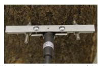
The DRW is the ruggedized version of the DR dendrometer type. In addition to the features of the simple DR version, the DRW dendrometer is modified for the use under especially harsh environmental conditions. A soft, weather-resistant rubber coating, protects the whole sensor from ingress of water and solid particles.
