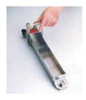
As the fluid flows down the instrument its progress can be accurately measured using the graduated scale. By comparing the flow rate to specified time periods the physical properties of the sample can be calculated.
