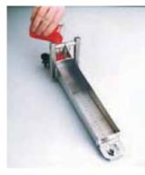
The gate is released, by pressing the lock release lever, while the spring action ensures it opens instantaneously.
