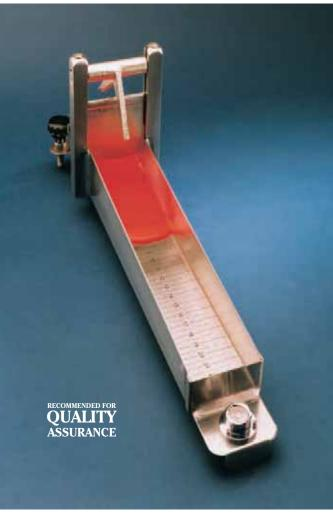
The Consistometer is a low cost, durable, instrument for accurately checking laboratory or production samples against consistency, viscosity or flow rate standards.
