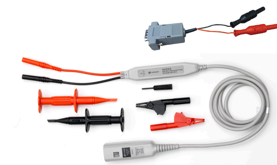
Figure 8. Keysight's N2818A 200-MHz differential active probe for CAN and FlexRay measurement applications. The optional DB9-SubD probe head makes it easy to connect to your differential bus.
