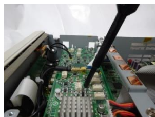
The measurement of conventional electric field probe
