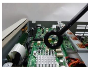
The measurement of conventional magnetic field probe
