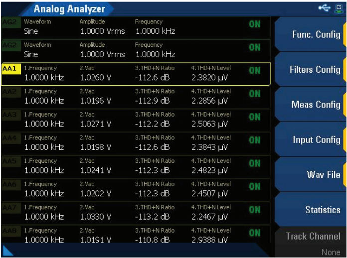
Figure 4. The U8903B's GUI, showing 8 analyzer channel measurements.
