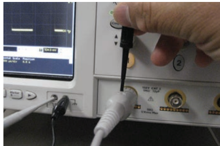
Figure 3-1. Use a small screw driver to adjust the probe's variable capacitance.
