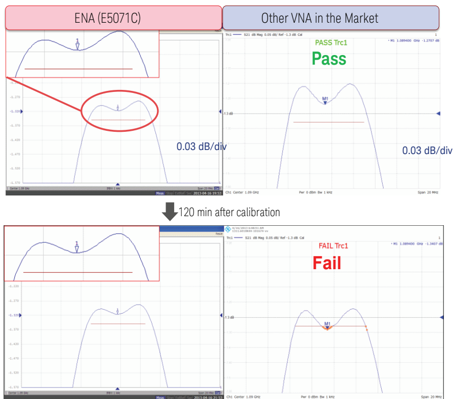
Figure 7. Stability comparison. Other VNA may incorrectly fail DUTs overtime due to temperature drift.
