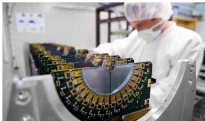
CERN - Assembling the last module of the vertex locator for LHCb. Photograph: Maximilien Brice. © 2007-2017 CERN. All Right Reserved.
