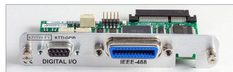
KTTI-GPIB GPIB interface with 6 digital I/O ports.
