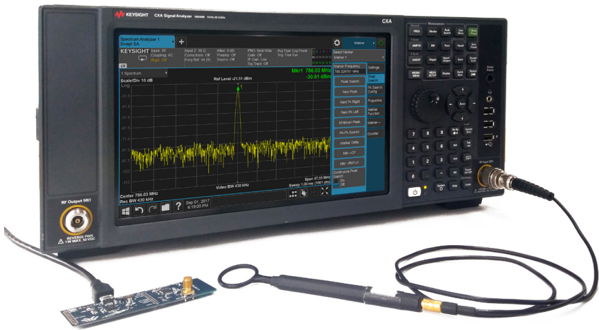
Near-field probe and CNA signal analyzer test the emission of PC LAN port during design cycle before full compliance testing.
