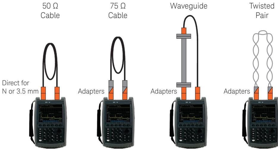
Figure 20. Test configurations for measuring other types of transmission lines
