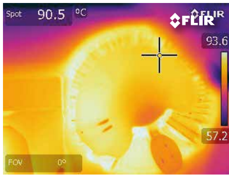
The PCB inductor is clearly visible in the thermal image through the PCB's epoxy layer.
