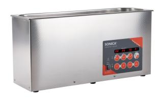
\* Stainless steel tank made in AISI 304 thickness 08/10 with round tank corners for a better removing of dirt residuals after cleaning process. The tank is conical and realized with a press machine
