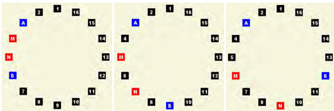
Electrode distance is one (left), two (middle) and three (right)
