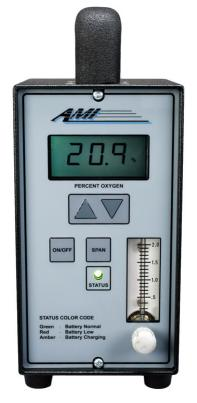
The AMI 111 series provide the ideal solution to percentage oxygen measurement in non-flammable gases. Most portable percent oxygen analyzers use replaceable electrochemical sensors, which suffer from drift, temperature and barometric pressure sensitivity, and require frequent replacement.
