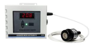
The Model 221R has become the standard oxygen deficiency monitor throughout the US market. It is used by the thousands in government labs, universities, and industry, anywhere there is a possibility of asphyxiation due to leakage of compressed or liquefied inert gases like nitrogen, argon or carbon dioxide.
