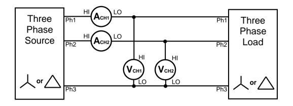
Three Phase Three Wattmeter - simulated neutral
