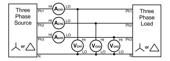
Three Phase Three Wattmeter – Star Connections
