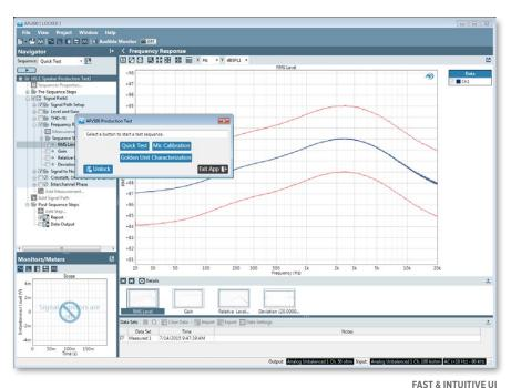
An example of the APx500 software's Production Test mode. In this mode, a test operator's use of the system is limited to a range of custom configurable presets.
