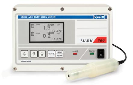
Basic kit Converting unit DH sensor Spare parts kit Calibrator Electrolyte Hydraulic panel HP 409 or flow-stabilizing module FSM 402 M Operation manual DH sensor DH 509 for the second channel Optionally Hydraulic panel HP 409 or flow-stabilizing module FSM 402 M
