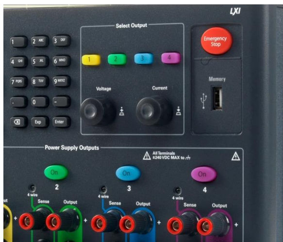
Figure 11. The N6705's front panel USB port.
