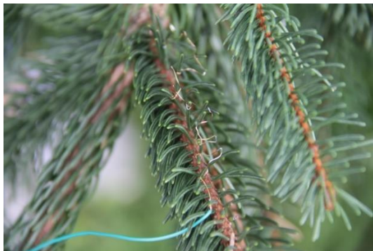
leaf temperature sensor type \Delta LA-C on Norway spruce
