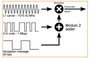
the carrier frequency. The carrier frequency for L1 is 1575.42MHz.
