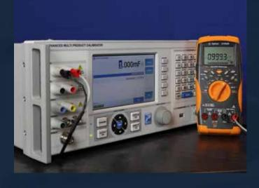
Included in -SYS units, the simulated option provides for resistance calibration between cardinal points and gives a continuous resistance range from 0 Ohms to 1 GOhms, with variable capacitance from 0.95uF through to 100mF.
