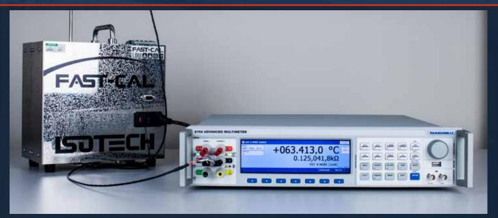
Included standard with the 8104 is the ability to measure temperature through 2, 3 and 4 wire PRT's and SPRT's with inbuilt support for both IEC 751 and ITS 90 probe coefficients. The 8104 displays both the calculated temperature and resistance simultaneously as well as the ability to ratio between two probes
