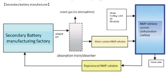
Installation point: Some measure NMP before they do concentration NMP solution (as you know NM-P&water), but most of them install at piping outlet after dehydration refining of rectification tower. (Blue section in above picture.)
