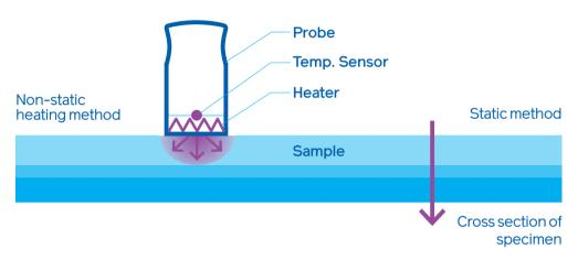
**Note:** For measuring the thermal conductivity of a non-homogenous or layered sample a device which uses the the static method is recommended.
