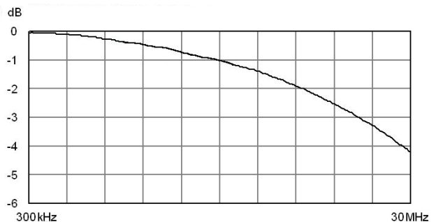
40-542-021 Insertion Loss Plot (typical worst case)
