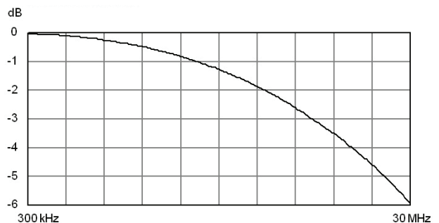
40-541-021 Insertion Loss Plot (typical worst case)
