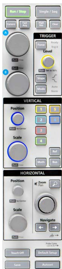
Figure 11: Efficient and intuitive front panel provides critical controls while still leaving room for the large high definition display.
