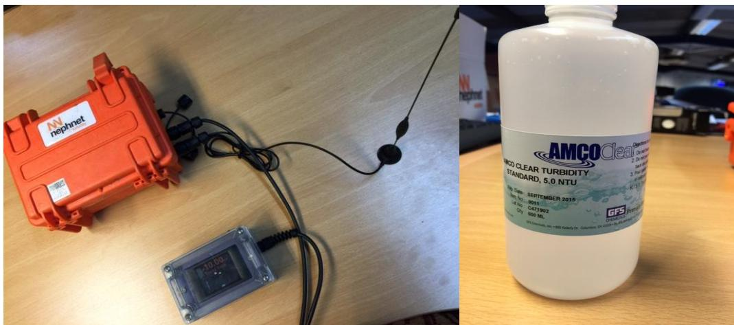
MAKE SURE THE UNUSED MILITARY SPEC'D CONNECTORS ARE SCREWED IN AND NOT LEFT LOOSE AS ABOVE. PLEASE ALSO MAKE SURE THAT WHEN CONNECTING, SIMPLY LINE THE PINS AND GENTLY PRESS AND SCREW IN AS TOO MUCH FORCE WILL BEND THE PINS
