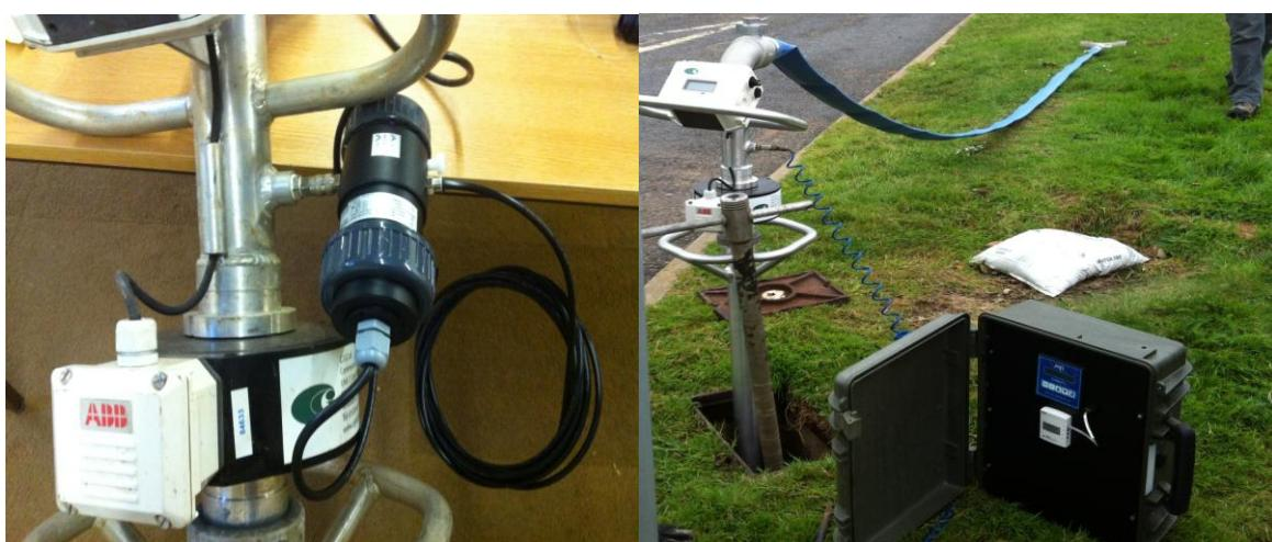
**Maintenance/calibration 'check' using a known standard or check 'block':**
