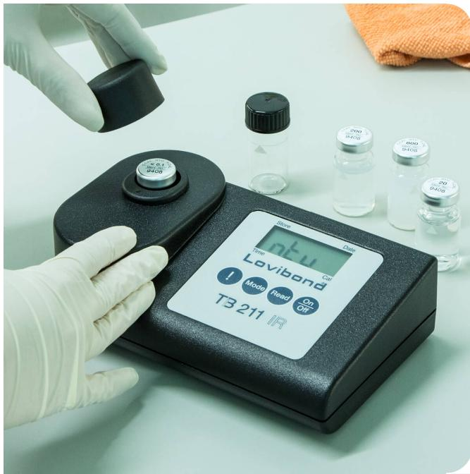
The compact Lovibond® infrared turbidity measuring instruments TB 211 IR & TB 210 IR for fast and accurate on-site analysis. It is measured as provided in EN ISO 7027, the scattered light at an angle of 90°.
